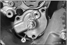
Using the oil pump sprocket bolt [A], pull out the oil pump
