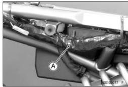
Remove the bolt [A], and lower the rear brake reservoir [B].
