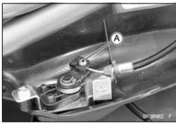
• Remove the quick rivet [A], and take off the rear fender.
