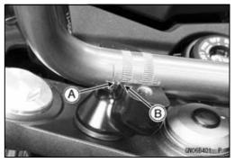
Tighten the front holder bolts first, and then the rear holder bolts. There will be a gap [A] at the rear part of the holder after tightening.
