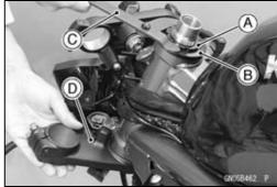
• To remove the ball bearing outer races [A] pressed into the head pipe [B], insert a bar [C] into the recesses of head pipe, and applying it to both recess alternately hammer it to drive the race out.
