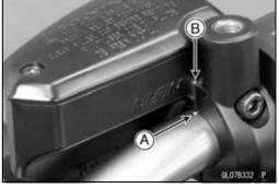
Tighten the upper clamp bolt [A] first, and then the lower clamp bolt [B]. There will be a gap at the lower part of the clamp after tightening.
