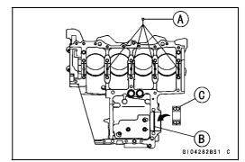
• Install the oil nozzles [A] in the upper crankcase, and tighten them.
