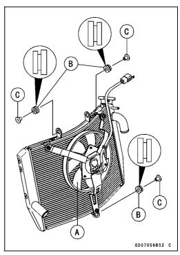
★ If the radiator bracket [A] was removed, install it.
