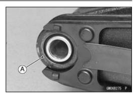
• Screw the adjusting collar [A] into the frame [B] so that the collar does not project the swingarm mating surface [C].
