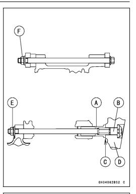
OSixth, tighten the middle engine mounting bracket bolts [A].
