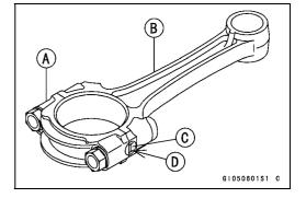
OWhen installing the inserts [A], be careful not to damage the insert surface with the edge of the connecting rod [B]
