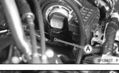
• Turn the headlight bulb [A] counterclockwise [B].
