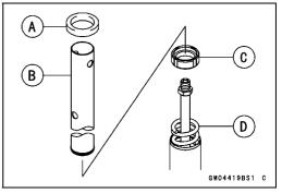
Remove: Damper [A] Spacer [B] Spring Joint [C] Fork Spring [D]
