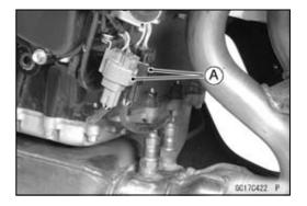
Set the hand tester [A] to the × 1 Ω range and connect it to the terminals in the oxygen sensor lead connector [B]. White Lead Terminal [C] White Lead Terminal [D]
