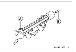
• Apply engine oil to the new O-rings [A] and the dust seals [B] of each injector.
