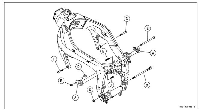
OThird, tighten the left upper engine mounting bolt [A]. [B] Frame
