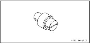
Bearing Remover Shaft,  $\phi$ 13: 57001-1377
