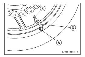
• Lubricate the tire beads and rim flanges on both sides with a soap and water solution or rubber lubricant. This helps the tire beads slip off the rim flanges.
