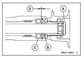
• Tighten the adjusting collar locknut [A] with the swingarm pivot nut wrench [B].
