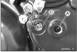
• Using a thickness gauge [A], measure the valve clearance between the cam and the valve lifter.
