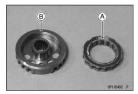
• Push [A] the starter clutch gear [B] in and turn it counterclockwise [C] and install it.
