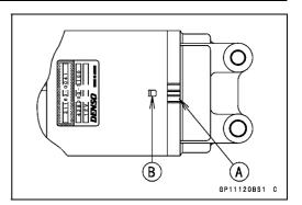
• Align the hollow mark [A] on the left-hand end cover and the hollow mark [B] on the yoke.
