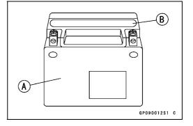
Terminal Voltage: 11.5 ~ less than 12.8 V
