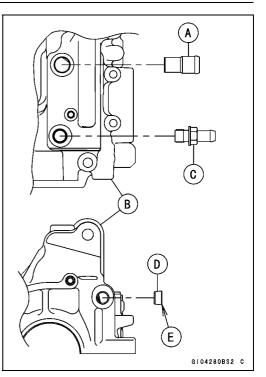
• Install the oil plugs [A] so that its surface is flush with the end of the hole.
