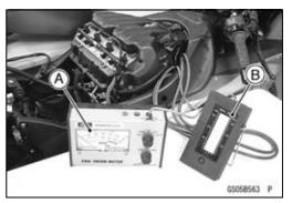
★ If any vacuum is not within the specifications, first synchronize the balance of the left (#1, #2 throttle valves) and right (#3, #4 throttle valves) assemblies.
