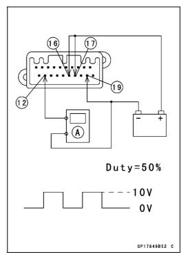
★ If each LED lights does not go on, replace the meter assembly.
