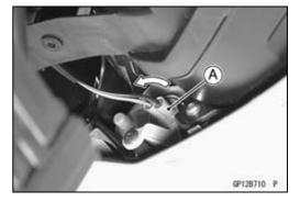
• Pull the bulb [A] out of the socket [B].
