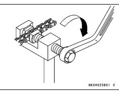
• Set the plate holder (b) [A] and cutting and riveting pin [B] as shown.
