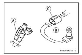
Olnjector signals can be also confirmed by connecting the hand tester (AC 10 V) instead of the test light set to the injector main harness connector. Crank the engine with the starter motor, and check to see if the hand oscillates at regular intervals.
