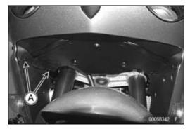
Remove: Quick Rivets [A]
