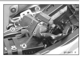
• Connect the hand tester [A] and 12 V battery [B] to the starter relay [C] as shown.
