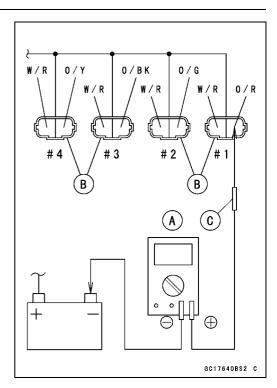
Primary Fuel Injector Output Voltage Connections to Injector #1 Meter (+)  $\rightarrow$  BL/R lead Meter (-)  $\rightarrow$  Battery (-) Terminal Connections to Injector #2 Meter (+)  $\rightarrow$  BL/G lead Meter (-)  $\rightarrow$  Battery (-) Terminal Connections to Injector #3 Meter (+)  $\rightarrow$  BL/BK lead Meter (-)  $\rightarrow$  Battery (-) Terminal
