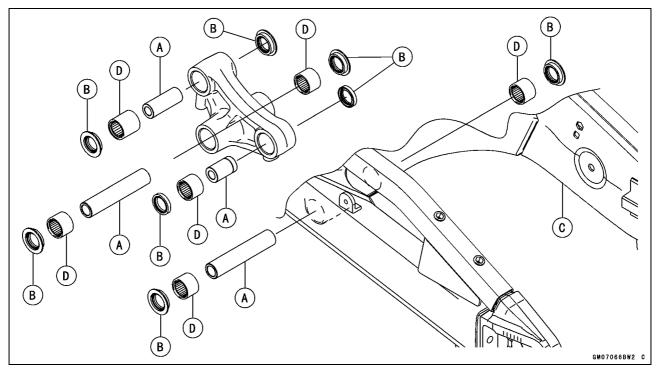
OWhen remove the needle bearings [A], tap the bearings evenly with the bearing remover shaft [B]. Special Tool - Bearing Remover Shaft,  $\phi$ 13: 57001-1377
