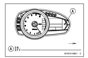
• Remove the key registration unit and connect the immobilizer/Kawasaki self-diagnostic system connector.
