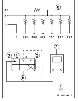
★ If the tester reading is not as specified, replace the gear position switch with a new one.
