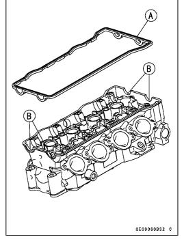
Be sure to install the following parts. Dowel Pins [A] Plug Hole Gaskets [B]
