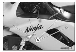
Remove: Quick Rivets [A]
