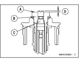
• Set the fork spring compressor on the spacer [A]. Special Tool - Fork Spring Compressor: 57001-1685
