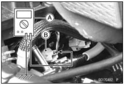
Secondary Fuel Injector Output Voltage Connections to Injector #1 Meter (+)  $\rightarrow$  O/R lead Meter (-)  $\rightarrow$  Battery (-) Terminal Connections to Injector #2 Meter (+)  $\rightarrow$  O/G lead Meter (-)  $\rightarrow$  Battery (-) Terminal Connections to Injector #3 Meter (+)  $\rightarrow$  O/BK lead Meter (-)  $\rightarrow$  Battery (-) Terminal Connections to Injector #4 Meter (+)  $\rightarrow$  O/Y lead Meter (-)  $\rightarrow$  Battery (-) Terminal
