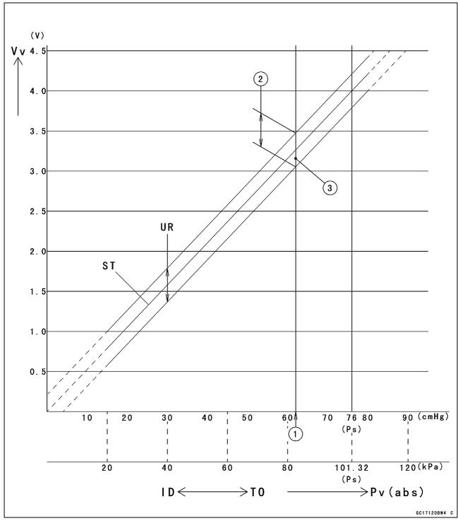
Inlet Air Pressure Sensor (Service Code 12)
