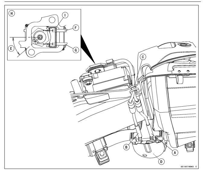
• Stretch the open cable (white) first by using the adjuster [A].
