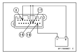
**Right and Left Turn Signal Indicator Light (LED)** Battery Positive (+) Terminal to Terminal [2] Battery Positive (+) Terminal to Terminal [10]
