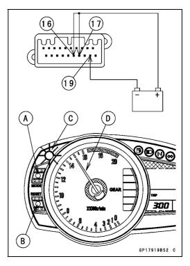
• When changing the pre-set engine speed, check that the tachometer meter needle moves (change of pre-set engine speed) within the adjusting range by pushing the RE-SET button.
